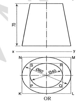
11 Draw the front view, side view from the right, and top view of the **10M** block as shown in figure (All dimensions are in mm)
